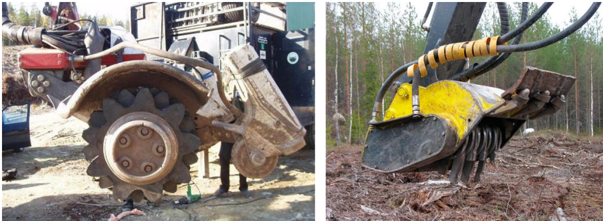
Figure 8. Crane-mounted devices for direct seeding that are no longer used: Humax (left) from Humax Forest AB in Hammerdal, Sweden, and Havel-rototiller from Havel Oy in Iломantsi, Finland. Poor soil preparation results were the main reason for discontinued use of both of these special devices (Nilsson 2009; Helenius & Saarinen 2013). Photo: Ida Nilsson and Pekka Helenius.
