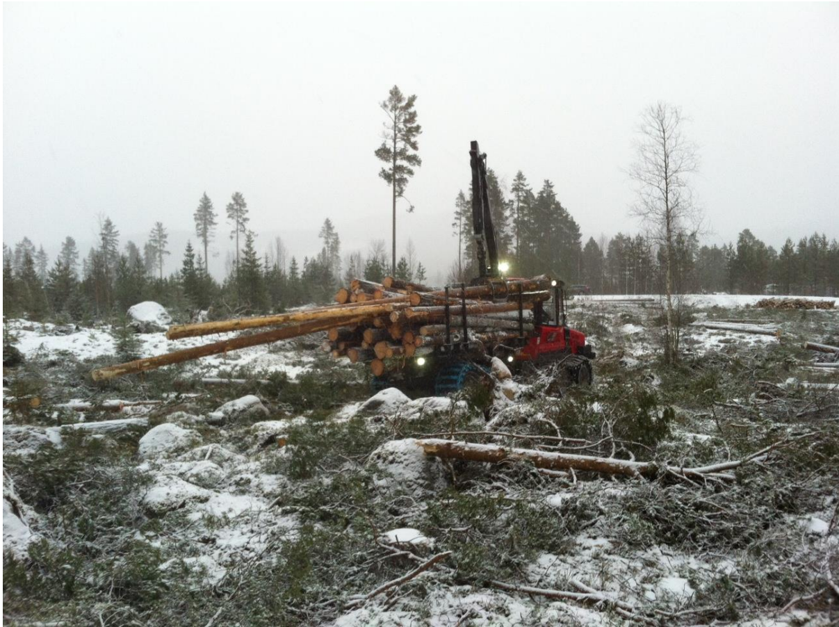
Figure 49: A large forwarder extracting sawlogs and two logs destined to become utility poles on a clearcut in northern Sweden (© Back Tomas Ersson, SLU).
