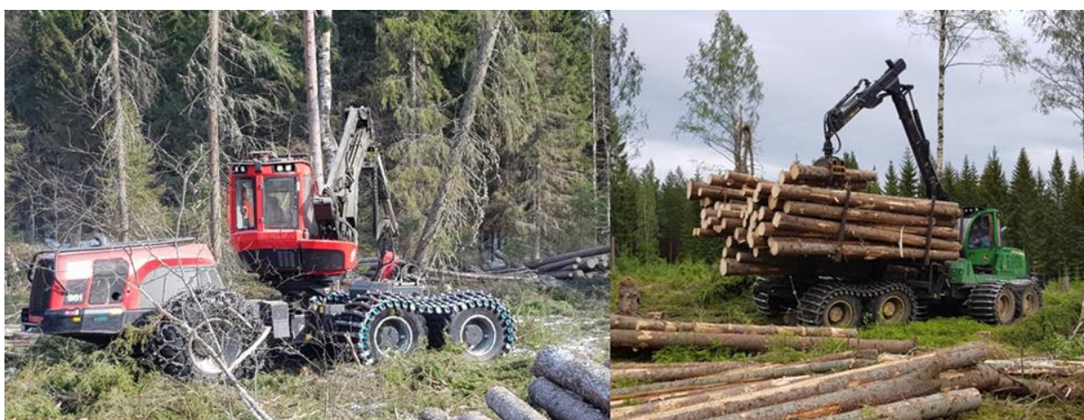
Figure 43: A harvester (left) and a forwarder (right) on final felling sites (© Tomas Nordfjell, SLU).
