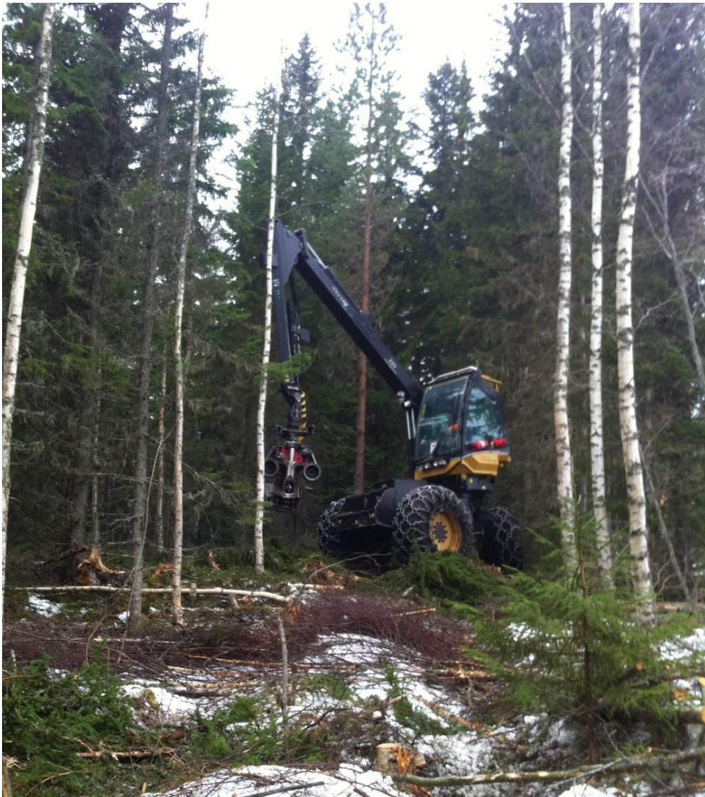
Figure 48: Commercial (first) thinning of a mixed conifer-deciduous stand using a small 4 wheeled harvester in northern Sweden in November 2017. Commercial thinning is performed yearly on over 300,000 ha in Sweden, Pulpwood is typically the main product produced during commercial thinning (© Back Tomas Ersson, SLU).
