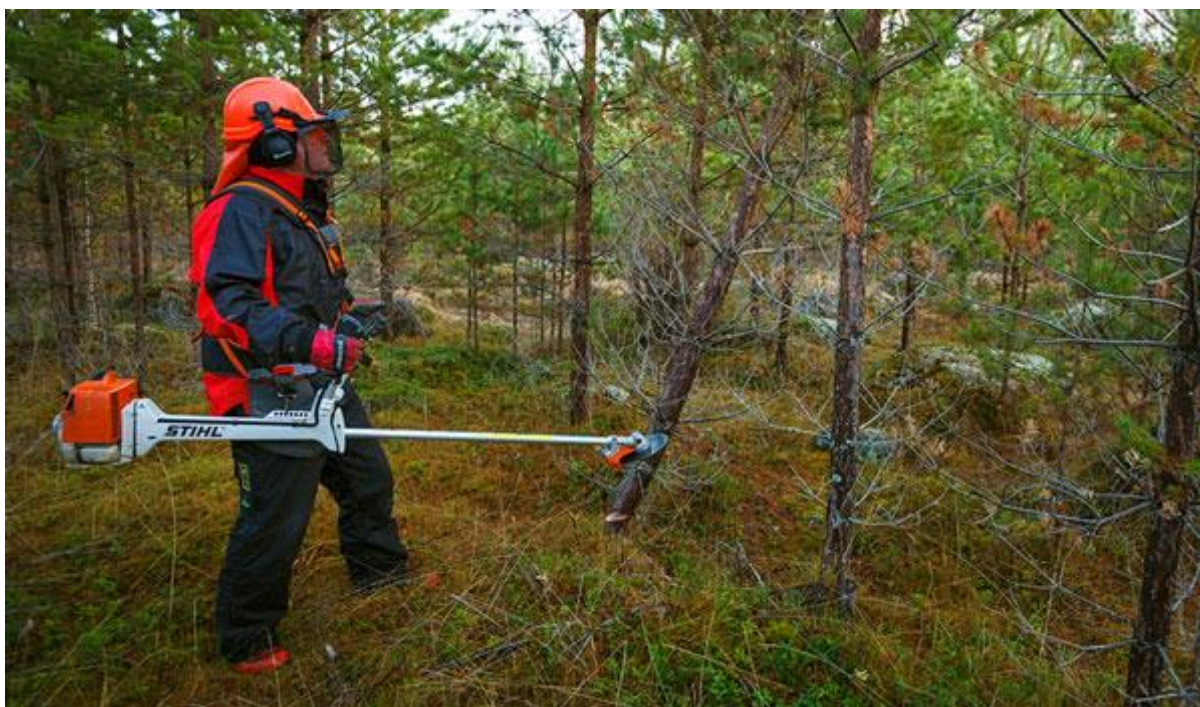
Figure 54: Motor-manual pre-commercial thinning (PCT) in a young pine ( Pinus sylvestris ) stand. PCT is a service commonly performed by contractors and bought by Swedish private forest owners from forest companies (© Stora Enso Skog).
