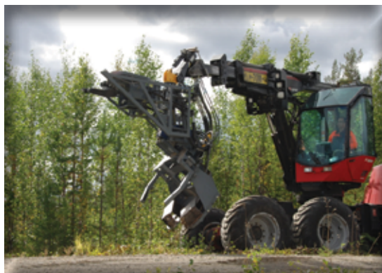
Figure 3. The pre-prototype boom-corridor felling head in an opened position (cf. Figure 2, right panel).
