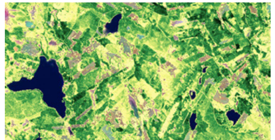
Subset of the stem volume layer in “Skogliga grunddata”. All of Sweden is covered with 12.5 m x 12.5 m raster data cells that show key forest variables for each cell.
