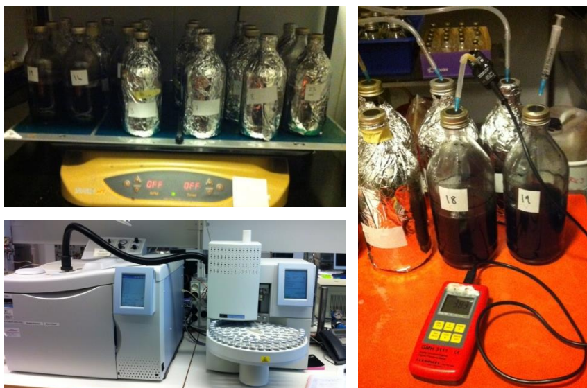
Figure 4. Bottles on the shake table at +37 °C and the gas chromatograph used for methane analysis to the left. To the right, monitoring of gas pressure and methane production.
