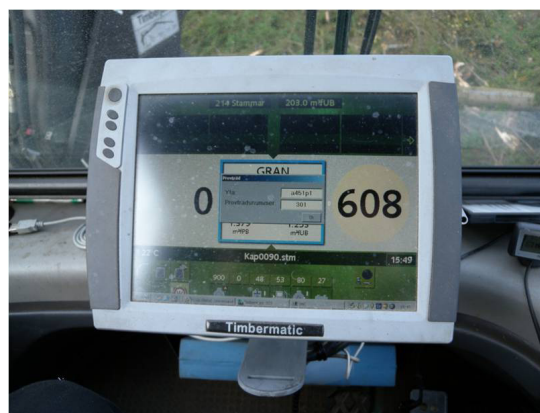
Figure 1. Ongoing research has shown the possibility of using stem data collected by a harvester's computer in order to estimate timber assortments in similar stands that have not yet been harvested.
