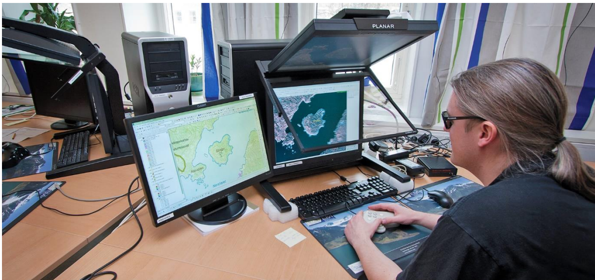
Figure 3: Photo interpreter performing manual interpretation at a digital photogrammetric workstation (Photo: Cronvall, 2012).
