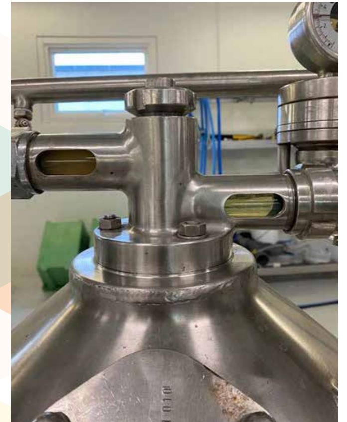
Fig. 1. Bulk centrifugation of precipitate from leaf juice at about 300L/hr. Incoming juice with precipitate on the left and precipitate free "brown juice" on the right. (Photo by William Newson).
