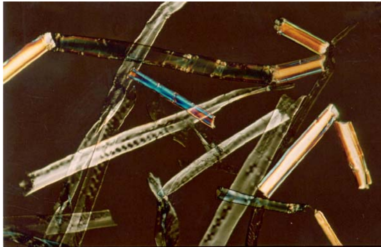
Figure 1. Cleavage of spruce earlywood and latewood pulp mill fibres by HCl after 4h at 80°C.
