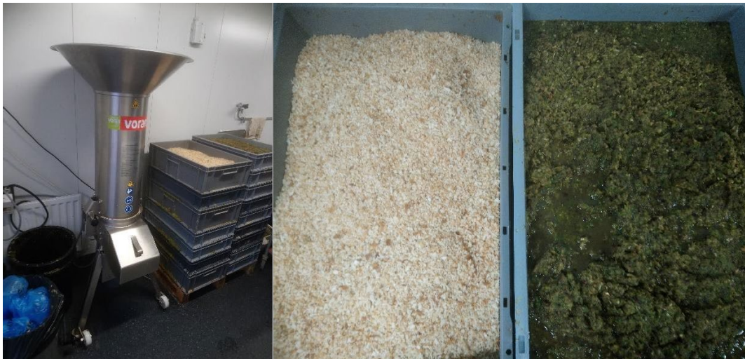
Figure 3. Picture of a) the milling machine; b) the milled bread; c) milled vegetables.
